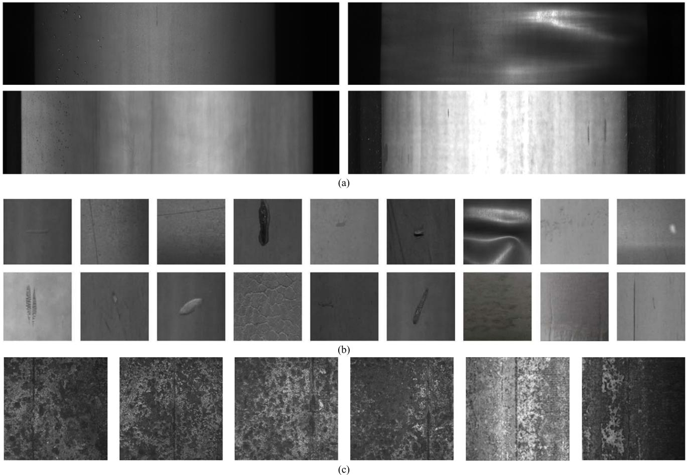
Fig. 2. Typical defect image samples. (a) Typical defective raw images of steel surface ( $4096 \times 1024$  pixels) acquired by line-scan camera and (b) series of typical defect samples with  $256 \times 256$  pixels for hot-rolled steel strips. (c) Typical longitudinal cracks acquired by area-scan camera for con-casting slabs.
