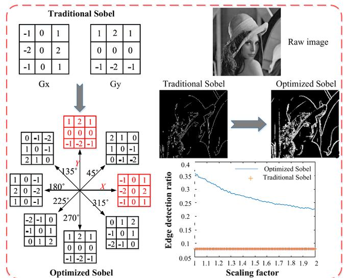
Fig. 4. Comparison of the traditional and the optimized Sobel operator.
