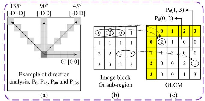
Fig. 5. (a) Direction analysis. (b) Image block. (c) GLCM of  $P_0$ .
