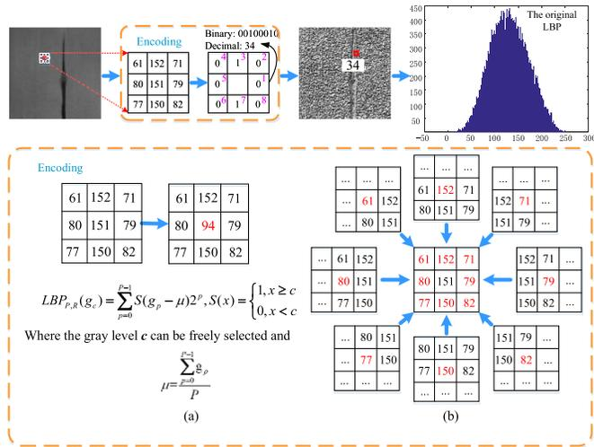
Fig. 6. Standard pipeline of original LBP and the variants of LBP based on changing threshold and scale. (a) LBP extension method based on changing threshold. (b) LBP extension method based on varying scale.
