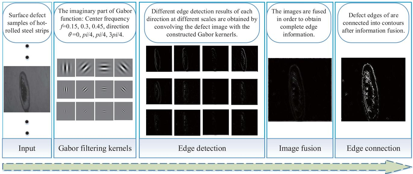
Fig. 7. Example of using Gabor filters to detect defect edges.
