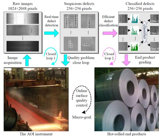
Fig. 1. Contribution of defect detection in a typical AVI instrument.
